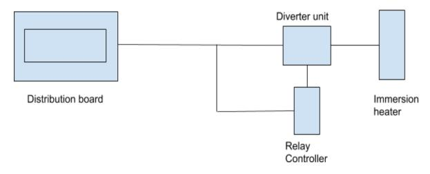
• In this case we are not switching the load ourselves but using the diverter to do it. We then control the diverter with our relay through inputs on the diverter.
